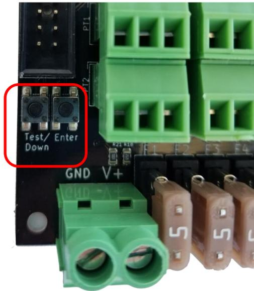
The button on the left is to navigate through the menu items or to display a test pattern if pressed from the Main screen. The button on the right is to select the highlighted item.
